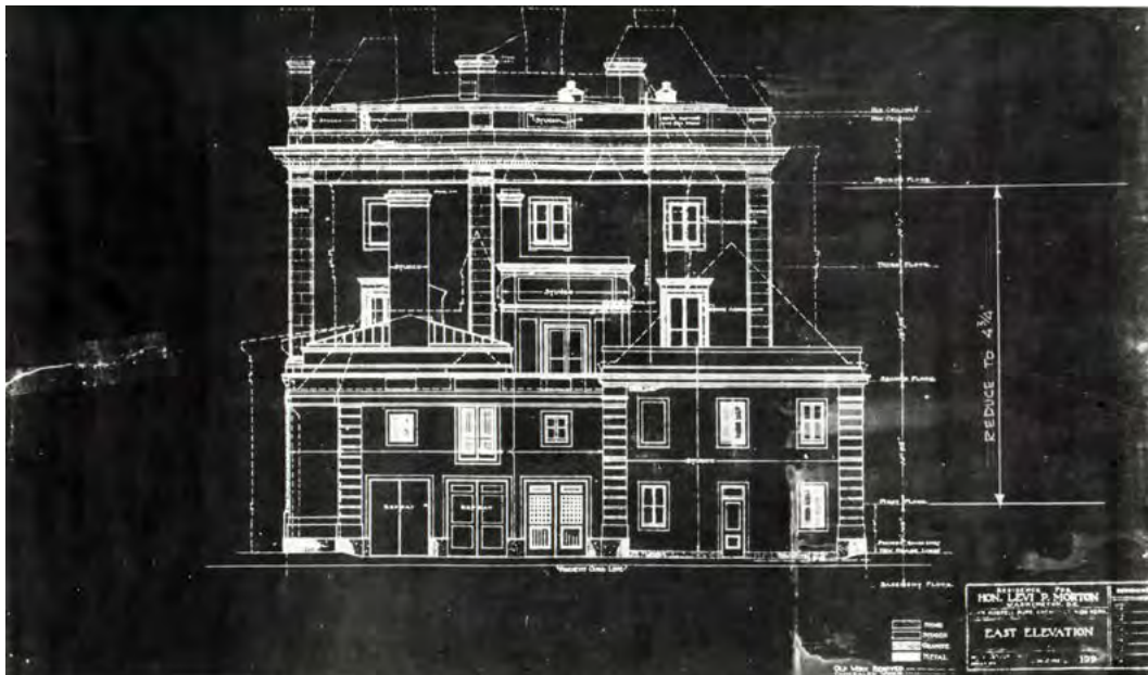
Figure 009 East elevation drawing of reconstructed residence, showing service wing with main block beyond, circa 1912. Silhouette of original house is dashed in beyond. U.S. Commission of Fine Arts, Vertical Files.
