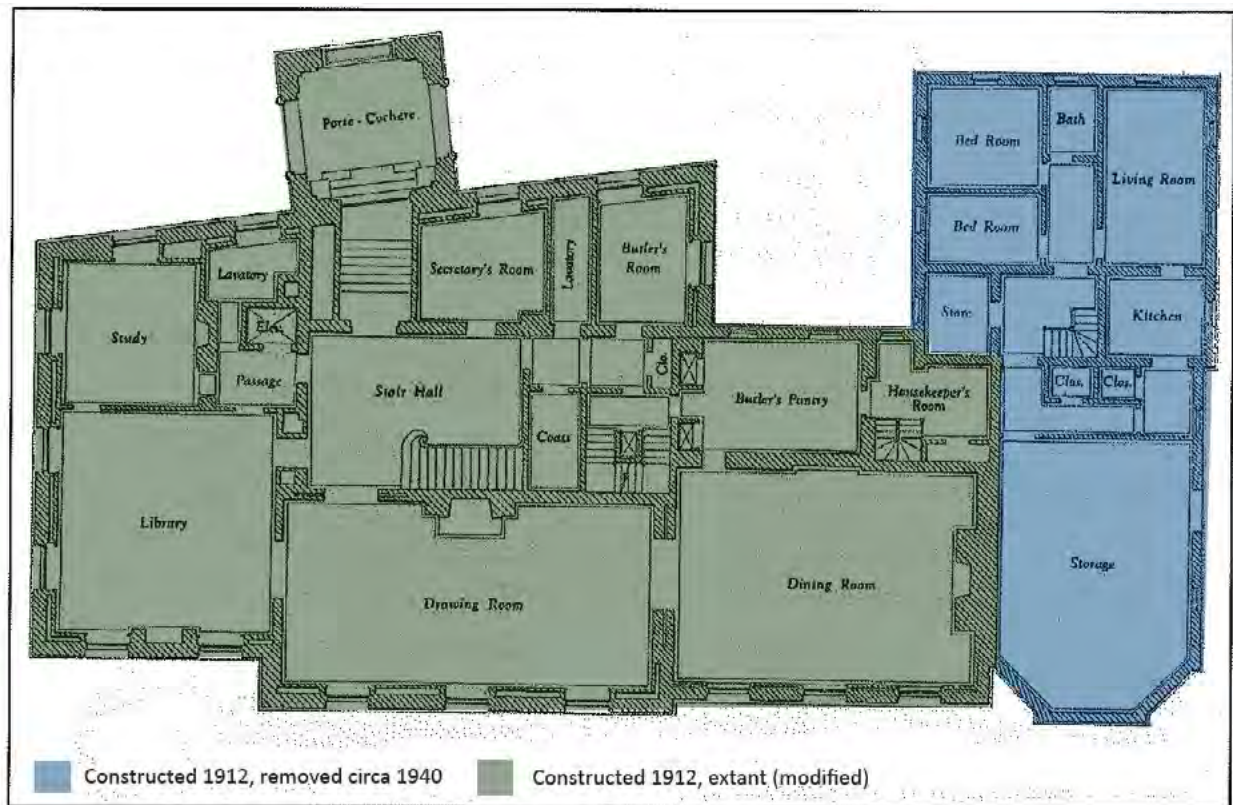
Figure 011 Plan of Pope's Reconstruction, circa 1912, showing garage and service wing removed circa 1940. U.S. Commission of Fine Arts.
